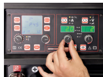
Welding thickness selection
