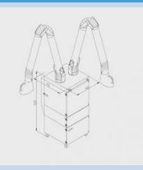
steels). If you handle the unit correctly, you can use it for circulating air operation because it fulfils the requirements for the exceptional rules according to the new German Hazardous Substances Ordinance. A baffle plate serves to pre-separate gross particles. Afterwards, the filter cartridge separates the
