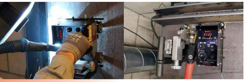
The Wel-Handy Mini Strong is a compact design welding carriage designed to perform horizontal, vertical, and overhang welding. A 35 kg magnet and 16 kg traction power provides reliable performance and quality welds. The machine is easily carried around with the handle with magnet detachment mechanism.
