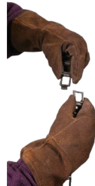
Chain links can be adjusted easily for various pipe diameters.
